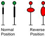
Note: Switch targets may be different shapes than illustrated but must not be diamond shape.
