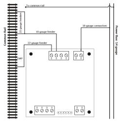
good practice to have a feeder for each section of track, even when track joints are soldered), or where the distance from the track connection to the card are longer, using an 18 gauge feeder from the card to a close location to the track is recommended.
