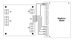
By default, changes to inputs do not send messages to LocoNet. Consult the DS64 instructions on setting Option Switch 13 to "Closed".
