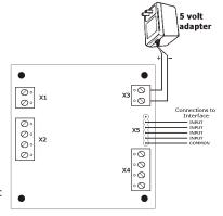
Your own power supply can be as simple as a DC wall adapter (a "wall wart", as they are sometimes called). Its current output should be capable of powering all the Quad Occupancy detectors it will supply. Each indicator can draw up to 10 mA (40 mA if all are on at the same time), though with a 5 volt supply, each will only draw about 2 mA (8 mA when all are lit).
