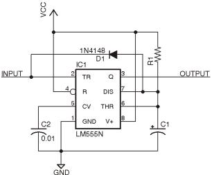
the timer period ends. Anytime the input returns low during the timing, the timing is halted and the output remains active. The next time the input goes high, the timing starts once again. The time duration is approximately equal to 1.1 times the product of R1 (in Ohms) and C1 (in Farads). For instance a 47 k $\Omega$  resistor and a 4.7  $\mu$ F capacitor provides a delay of just under 0.25 seconds.
