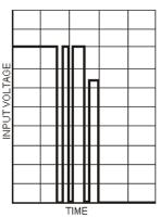
With an occupancy detector, bounce is magnified by track conditions. Slightly dirty sections of track can add to bounce noise. Momentary loss of detection can even be substantial enough to have an effect when driving a relay circuit. The Quad Occupancy Detector from Circuits4Tracks counters the effects of momentary loss of detection with the use of a capacitor on its output, but bouncing will still occur when the state changes from unoccupied to occupied and back again.
